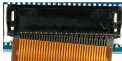
FPC is inserted diagonally.
